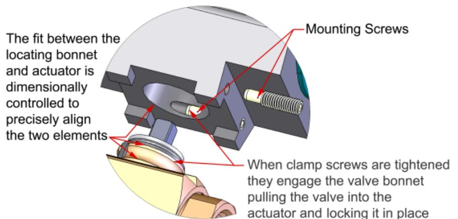
absorbed independent of the clamp screw by means of a four corner mounting pad that straddles a mating projection on the valve body. This locks the
